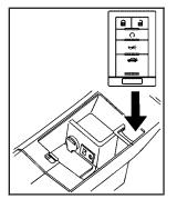
If moving the transmitter to different locations within the vehicle does not help, place the transmitter in the center console transmitter pocket with the buttons facing to the right and then press the START button.
